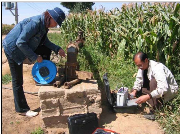
Measuring water level and flow rate at a production well in Chahaertan oasis
