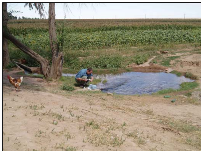
Sampling groundwater from a well outlet pipe to an irrigation pond, showing the contrast between sandy un-irrigated soil in the foreground and irrigated sunflower and maize fields behind
